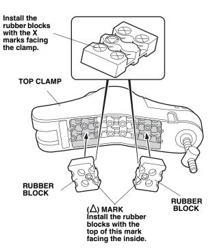
Install the rubber blocks with the top of this mark facing the inside.
